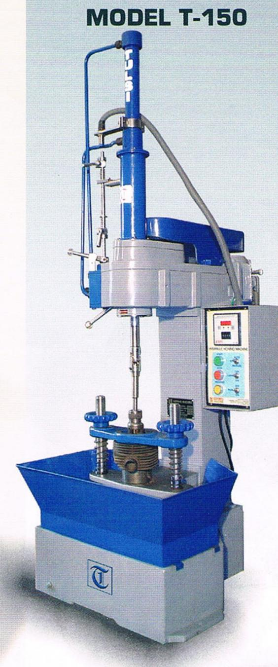
Honing is a super finishing process, which has all the importance in Cylinder Block reconditioning. A perfect hatch angle has to be maintained as per the recommendations of the manufacturer to ensure efficient working of the engine and reduce oil consumption in a re-conditioned engine.
